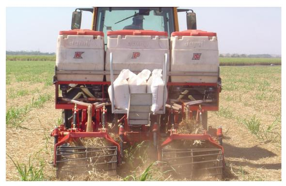
Cultivation sugar cane trencher, fertilizer and cultivator applying 3 inputs at the same time with variable rates.
